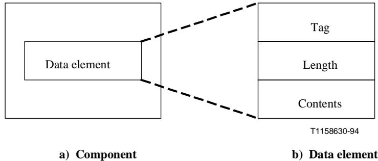
**Figure III.1/Q.932 – Structure of component and data element**
