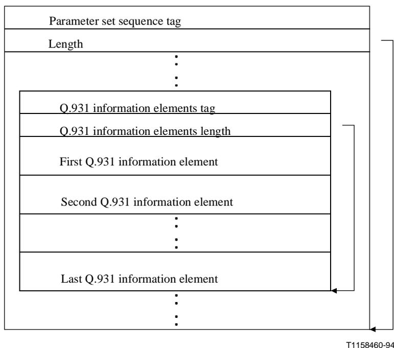
**Figure 8-4/Q.932 – Encapsulation of Q.931 information elements**
